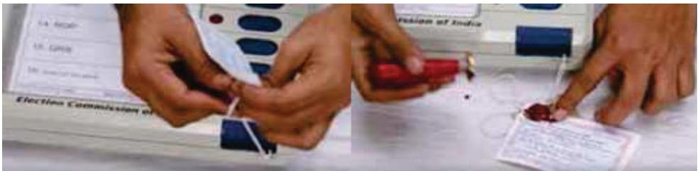
After unmasking candidate buttons, seal the upper cover of the BU by thread passed through holes on the top and bottom end at right side using address tags showing the particulars of the election with the seal of the RO.
