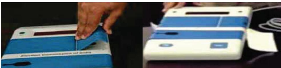
After Candidate set, seal cover of the Candidate Set Section and Battery Section of CU by passing a thread through hole provided on the respective side using address tags showing the particulars of the election with the seal of the RO.
